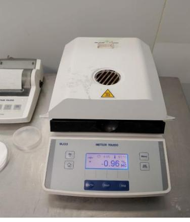
A white IR desiccator with a digital display showing '-0.96' and a keypad. The brand name 'METTER TOLEDO' is visible.          |
